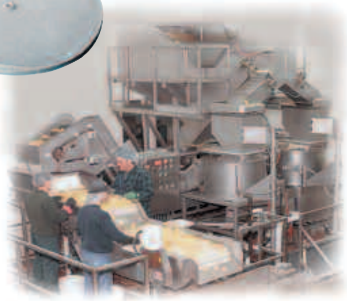
Custom systems are available with two-stage batch peelers, dewatering hoppers, diverting chutes, inspection/trim conveyors and platforms.
