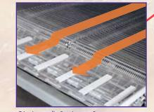
Discharge/infeed transfer conveyors prevent product damage during transfer. Lecithin applicator is available on infeed belt to reduce product sticking.
