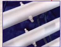
Clean-in-place sprays are built into the conveyor support framework to thoroughly clean both sides of the belt.
