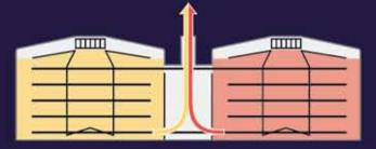
On two-zone models, venting exhaust through a central stack prevents the cooking atmosphere from migrating between zones. Steam only, dry heat, or any combination can be controlled independently in each zone without affecting the other zone.
